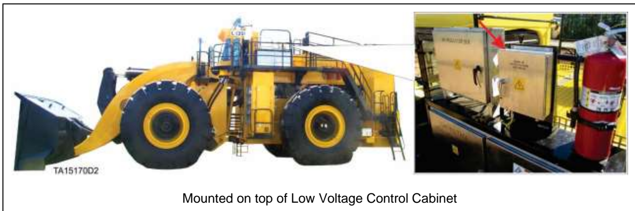
Figure 32. Engine air restriction indicator box (current machine models)
