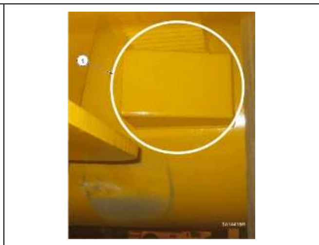
Figure 35. Typical axle vent
