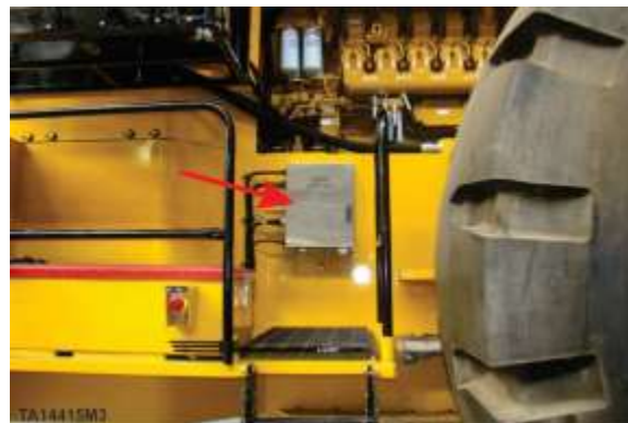
Figure 20. Typical engine interface box and typical locations
