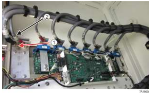
1) Positive bus bar, 2) Negative bus bar
