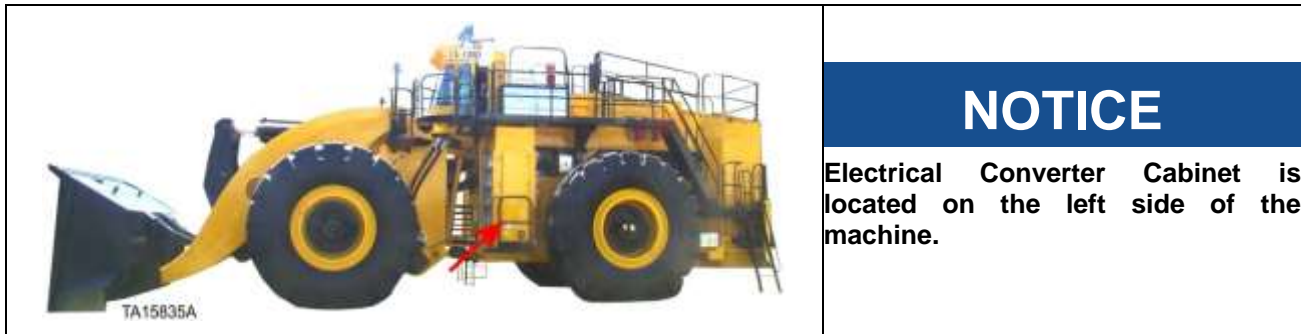
Figure 24. Electrical converter cabinet (typical)
