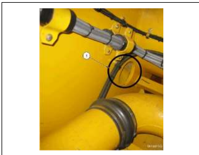
Figure 34. Typical axle vent front frame
