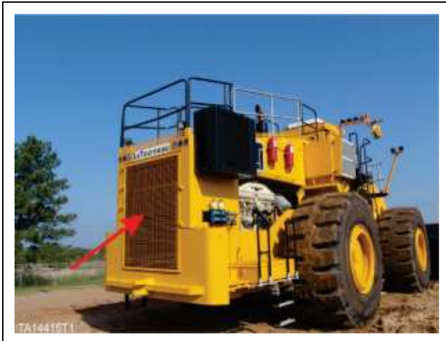
Figure 22. Rear frame (typical)
