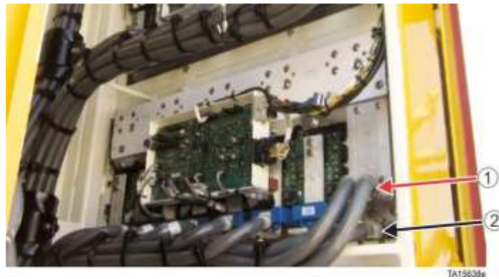
1) Positive bus bar, 2) Negative bus bar
